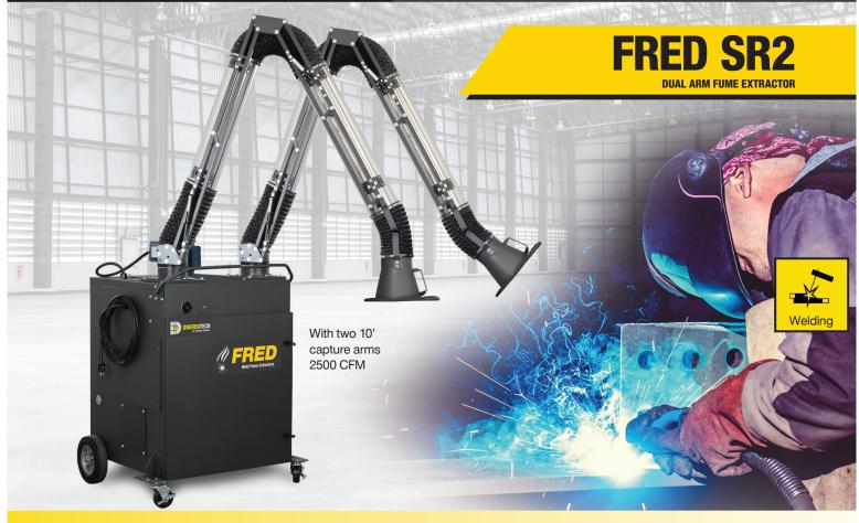
This professional grade fume extractor is the industry standard for eliminating smoke, dust and other unbreathables from the air. A 2500 CFM, 5HP blower ensures a high face-velocity across two independently movable capture arms, removing particulate as small as 0.5 micron with our standard MERV 15 rated Nanofiber filter.
